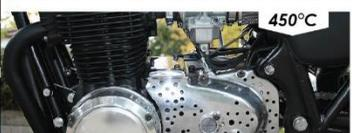
The coating contains specific silicone-based enamel which can withstand extreme temperature.
